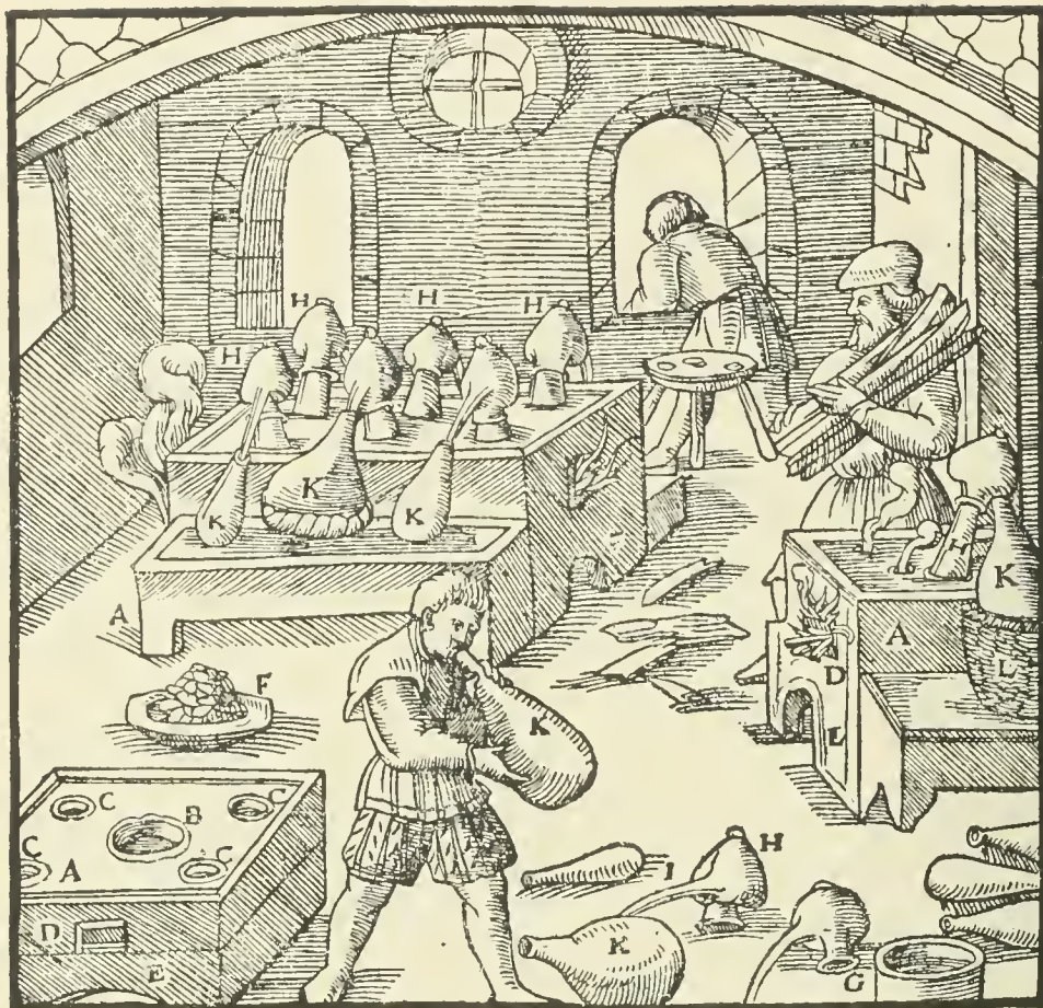
A—FURNACE. B—ITS ROUND HOLE. C—AIR-HOLES. D—MOUTH OF THE FURNACE. E—DRAUGHT OPENING UNDER IT. F—EARTHENWARE CRUCIBLE. G—AMPULLA. H—OPERCULUM. I—ITS SPOUT. K—OTHER AMPULLA. L—BASKET IN WHICH THIS IS USUALLY PLACED LEST IT SHOULD BE BROKEN.
